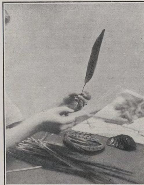
MONTAGE DE LA PLUME SUR LAITON
